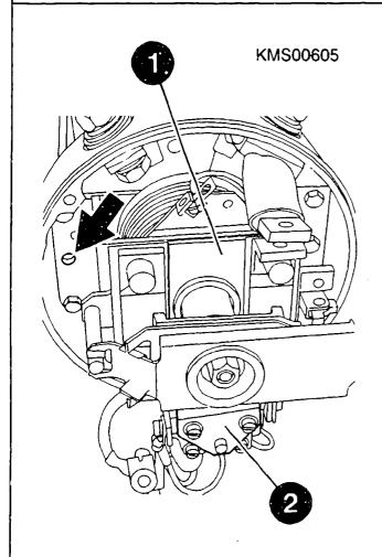
Unfasten bolts of starting-motor solenoid and detach starting-motor solenoid together with control relay.
